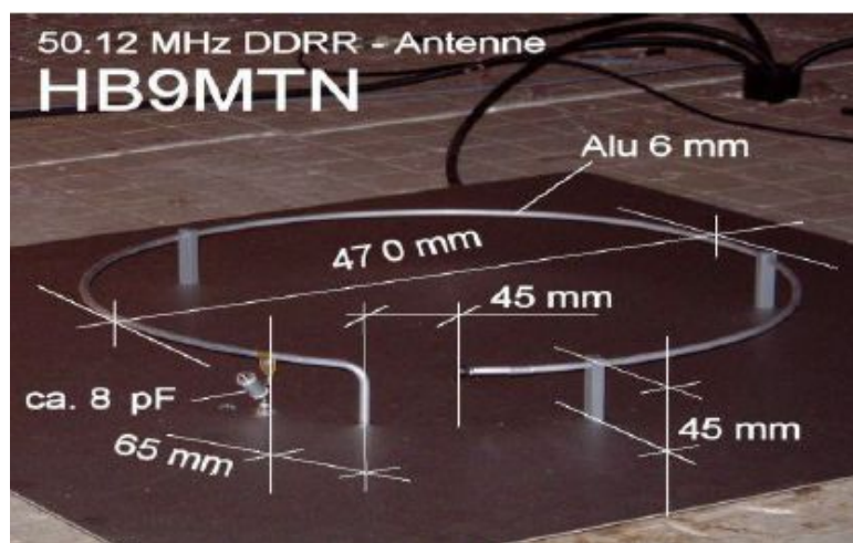
DDRR implementation for 50MHz
